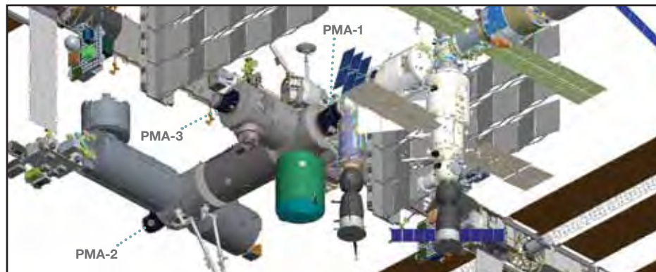
PMA-1 is being attached to the Common Berthing Mechanism of Node 1.
