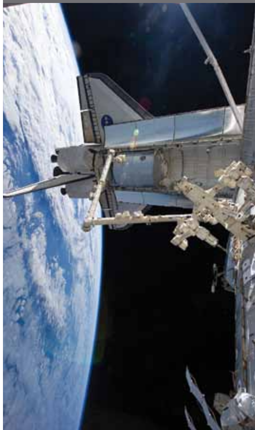
The station's robotic Canadarm2 grapples the Leonardo Multi-Purpose Logistics Module (MPLM) from the payload bay of the docked Space Shuttle Discovery (STS-131) for relocation to a port on the Harmony node of the ISS. Earth's horizon and the blackness of space provide the backdrop for the scene. Canadian-built Dextre, also known as the Special Purpose Dexterous Manipulator (SPDM), is visible at bottom center.
