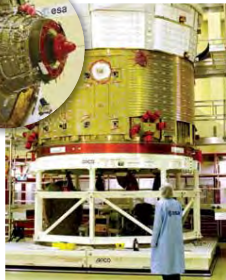
The ATV during manufacture.
