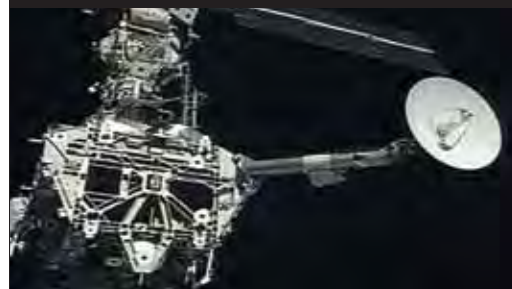
Ku band radio on exterior of ISS.
