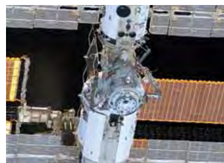
Pirs Module location at Service Module nadir.
