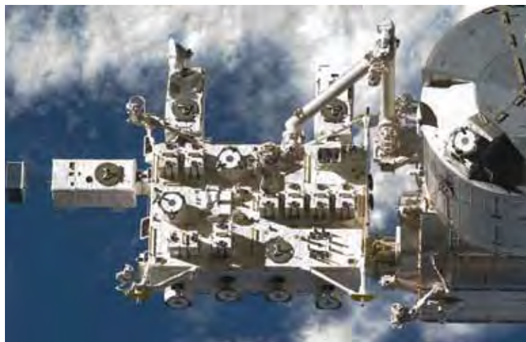
Japanese Experiment Module External Facility (JEM EF) with the Remote Manipulator System arm and three payloads installed.
