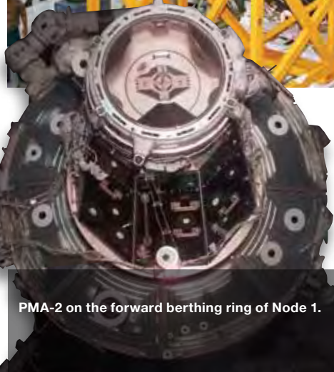
PMA structure shows a series of offset aluminum cylinders.
