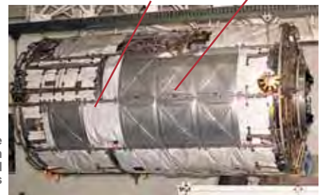
Intermediate Debris Shield, Nextel, and Kevlar Blankets. Outer Debris Shield, Aluminum
