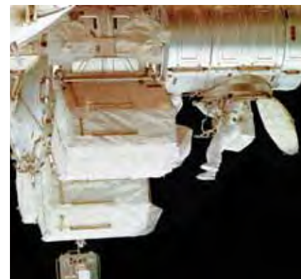
Crewmember entering the airlock extravehicular hatch.
