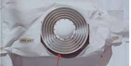
GPS antenna on S0 Truss.
